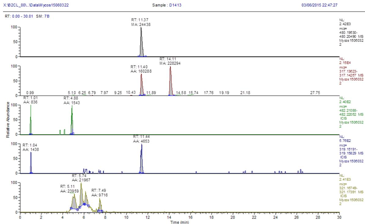
Peaks from top to bottom: 1. ZEN-4-Sulf, 2.  $\alpha/\beta$ ZEL-Sulf and ZAN-Sulf, 3.  $\alpha/\beta$ ZAL-Sulf, 4. H-ZEN, 5. DHZEN, 6. ZOM-1
