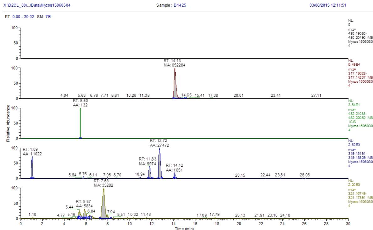
Peaks from top to bottom: 1. ZEN14SulfS, 2.  $\alpha/\beta$ ZEL14Sulf and ZAN-Sulf, 3.  $\alpha/\beta$ ZAL-Sulf, 4. H-ZEN, 5. DHZEN, 6. ZOM-1
